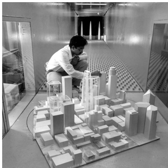
Figure 3: Photograph of model of downtown Minneapolis on a turning table in the SAFL boundary layer wind tunnel.
